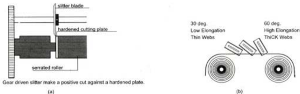
Figure 2: Slitting blade should not have any runout. Or the blade holding should be correct. Otherwise, uneven edges will be trimmed.
