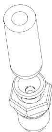
Figure 3: Air Gun Nozzle for Filling Air in the Air Valve. Keep it pressed for Air inflation.
