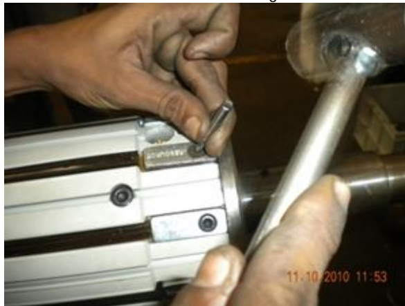
Figure 10: Loosen the CSK with center Punch, if not able to open with Allen key.
