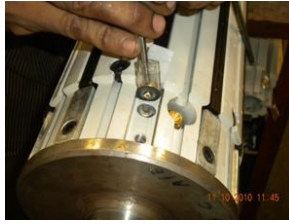
Figure 8: Thin Black Washer to be mounted.
