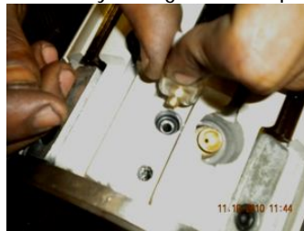
Figure 6: Inserting O-ring in the shaft.
