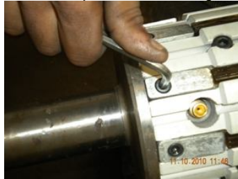
Figure 9: Loosen the Lock Piece
