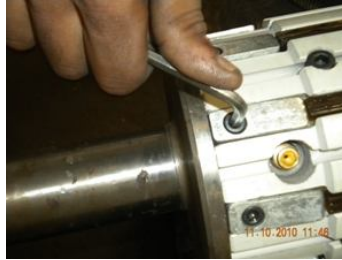
Figure 4: Loosen the Lock Piece
